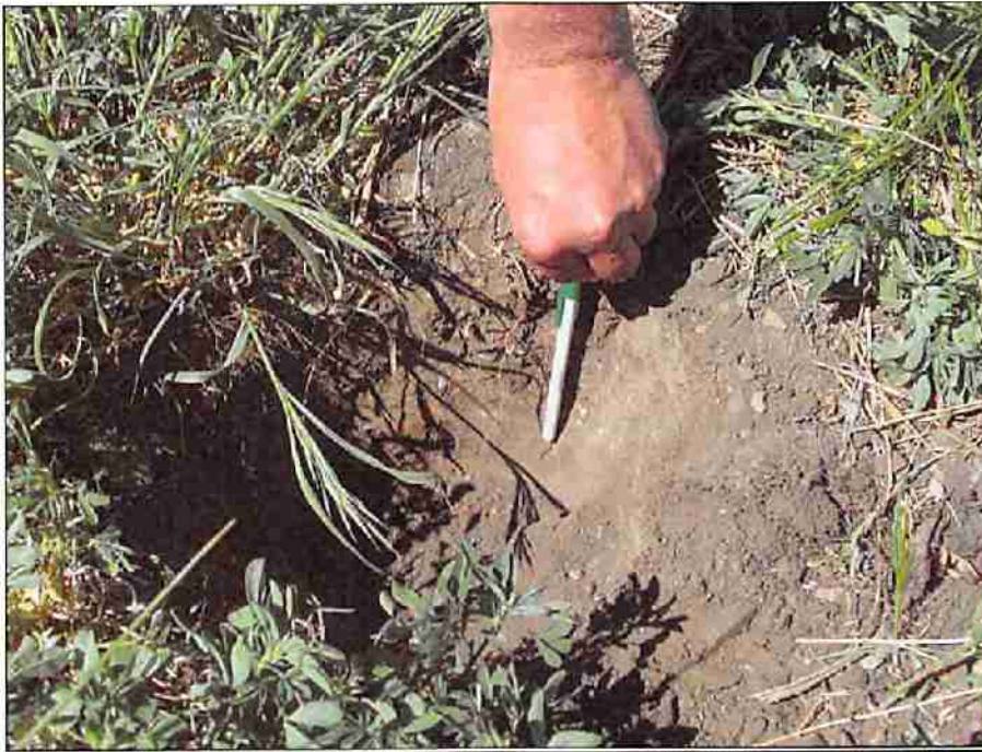
Photo 2: Topsoil depth on undisturbed areas (approx 20 cm).
