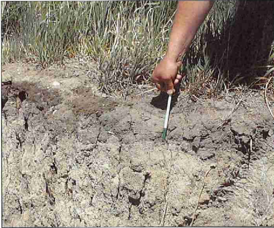
Photo 5: Looking at topsoil depth at northern pit face (approx. 20 cm).
